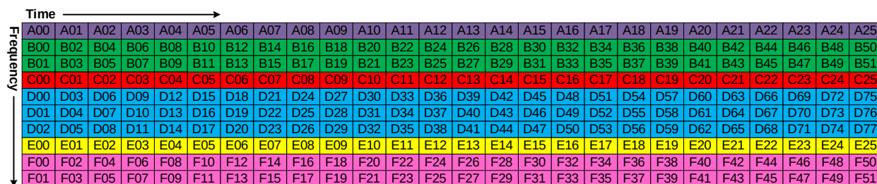
Figure 7.24 Example of frequency division multiplexing of PLPs.
