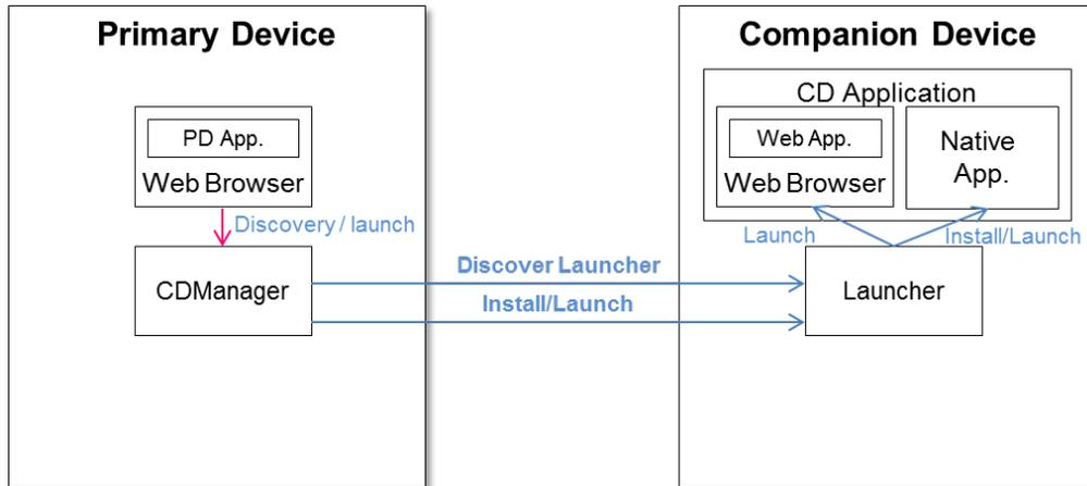
**Figure 5.1** Architecture for launching a companion device application.
