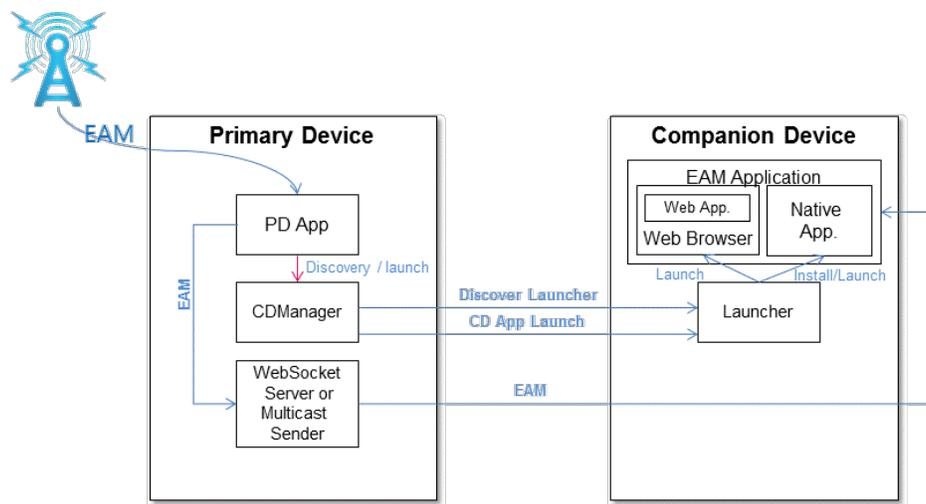
**Figure 5.4** Architecture for CD application to PD communication.
