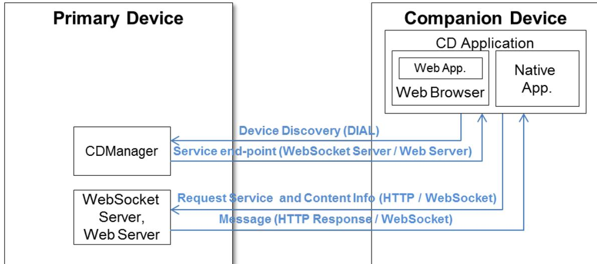
**Figure 5.3** Architecture for CD application to PD communication.
