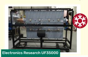
ERI Model UF35000-86 8 Section Reflective UHF Band Pass Filter System integrated with an output directional coupler, panel and system test load.
