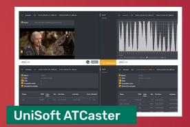
S&T's ATCaster generates ATSC3.0 ROUTE signaling and content over UDP output. It provides a complete ATSC 3.0 transmission chain when combined with AV encoders, schedulers and exciters.
