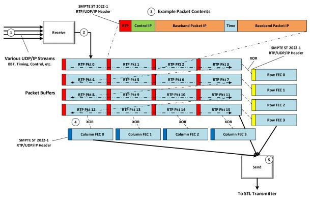
Figure 8.2 Example FEC encoding process diagram.
