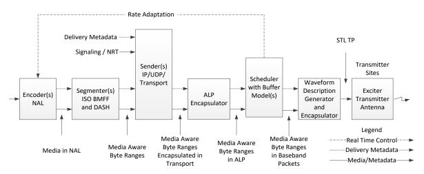
Figure C.1.1 Cascade of real-time functions involved with Scheduler.
