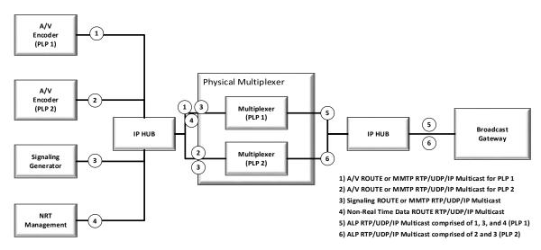
(SSM) and all Network connections can be accomplished with relatively inexpensive hubs or switches.
