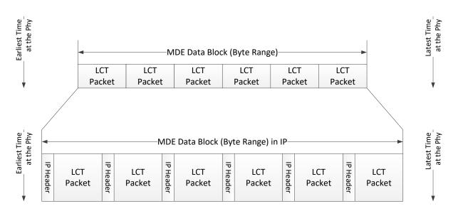
Figure C.1.6 Relationship of an MDE in LCT packets to IP encapsulation.
