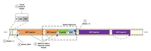
Figure 8.3 RTP Encapsulation example diagram.
