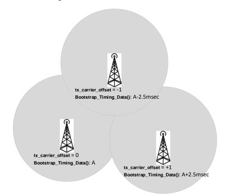
Figure 9.1 Example use of carrier and timing offsets for neighboring co-channel stations.
