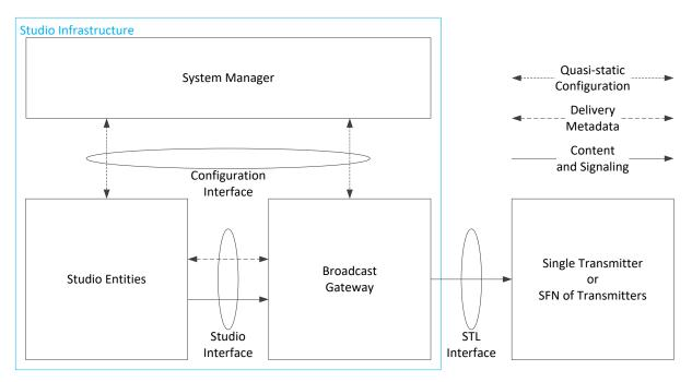
Figure 1.1 In-scope interfaces description.
