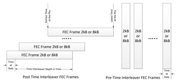
Figure C.1.3 Illustration of Earliest and Latest Time with a block interleaver.
