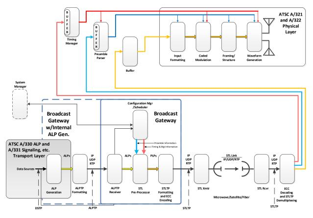
Figure 4.1 High-level overview of system configuration.
