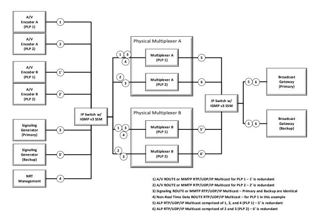
Figure B.1.3 Fully redundant routing example.
