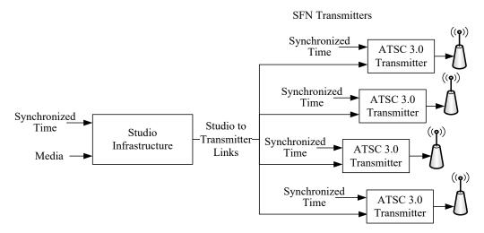
**Figure 5.2** System locations requiring synchronized time.
