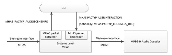
Figure A.4.2 Interface on systems level for user interactivity.
