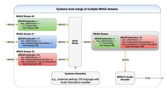
Figure 4.2 Example of switching and merging multiple incoming streams.
