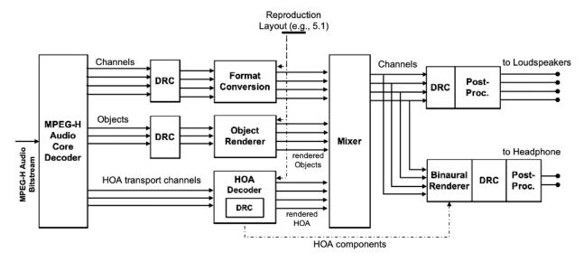
Figure A.1.1 MPEG-H Audio Decoder (features, block diagram, signal flow).
