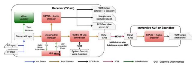
Figure A.6.1 Top level block diagram of a receiver using MPEG-H Audio.
