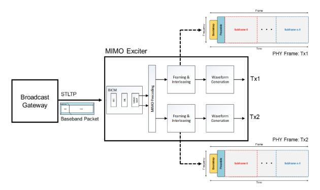
Figure F.1 MIMO Configuration in Broadcast Gateway and Exciter.
