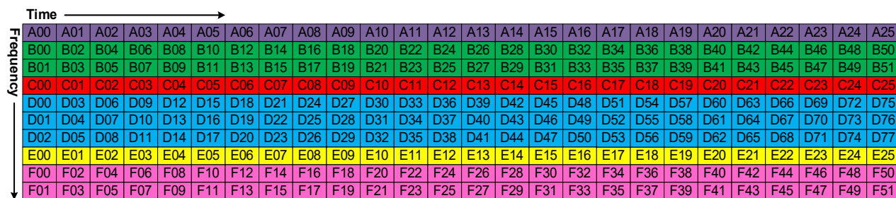
Figure 7.24 Example of frequency division multiplexing of PLPs.
