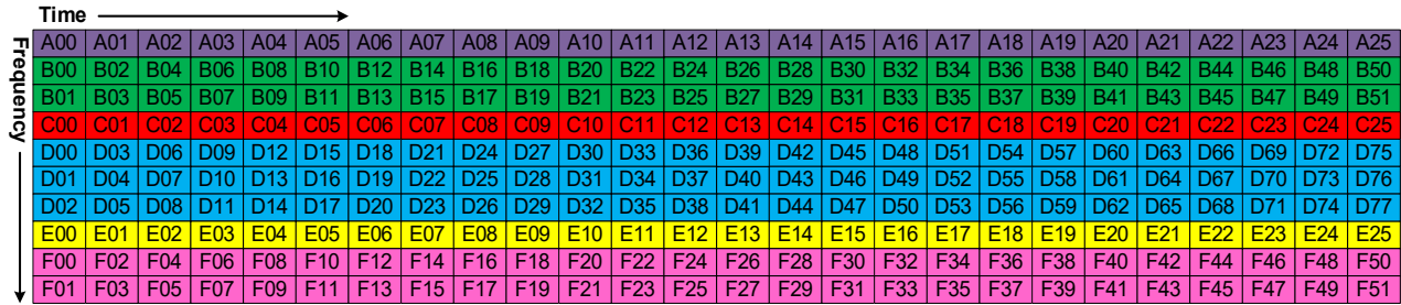
Figure 7.24 Example of frequency division multiplexing of PLPs.
