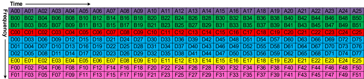
Figure 7.24 Example of frequency division multiplexing of PLPs.
