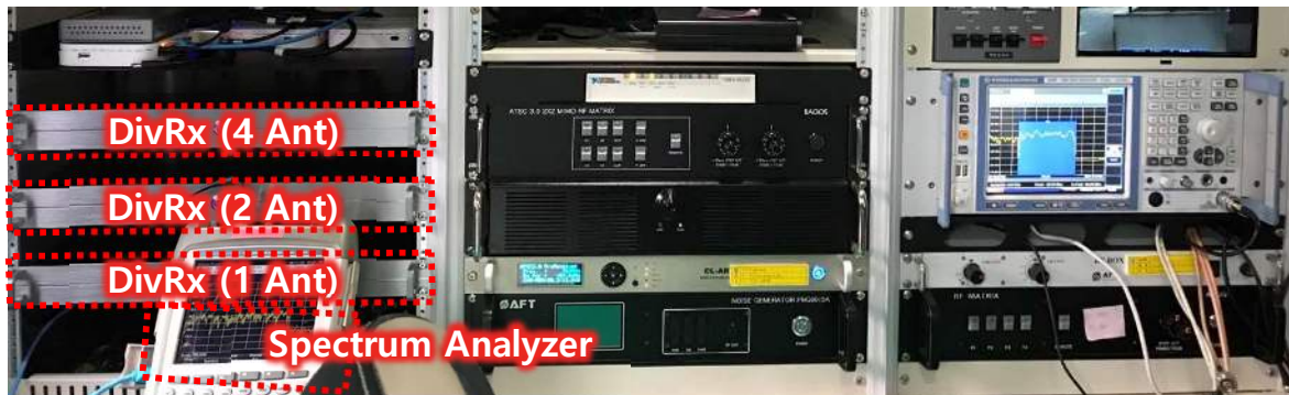
<Measurement Facility with Diversity Rx Sets>
