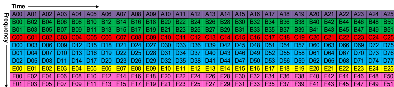
Figure 7.24 Example of frequency division multiplexing of PLPs.
