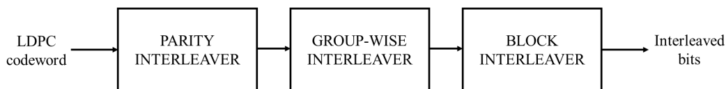
Figure 5.3 Bit interleaver structure: Parity, group-wise and block interleavers.
