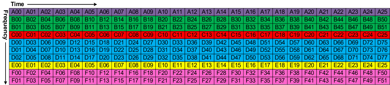
Figure 7.24 Example of frequency division multiplexing of PLPs.
