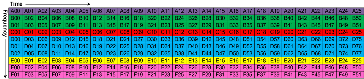
Figure 7.24 Example of frequency division multiplexing of PLPs.
